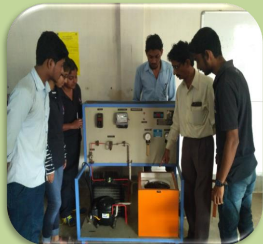
REFRIGERATION TEST RIG.
