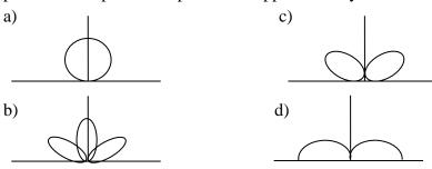
11. Two identical and parallel dipole antennas are kept apart by a distance of  $\lambda/4$  in the H – plane. They are fed with equal currents but the right most antennas have phase shift of +90°. The radiation pattern is given as(2)
